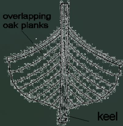
Viking longships were among the first ever ships to have a keel. The keel is extremely important as it provides the ship with support in rough weather.
